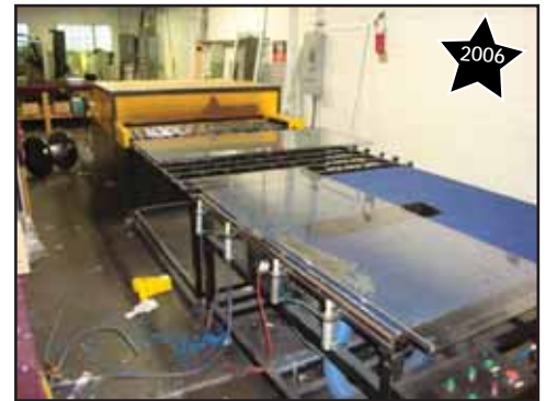
Stone Glass Drying Line
